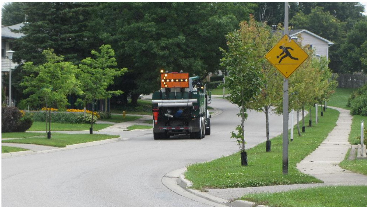
Figure 7: View of rear of truck with a TC-12 warning sign, with a arrow signally that approaching traffic should pass the truck on the left.
